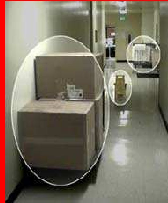
Obstructed exit route
